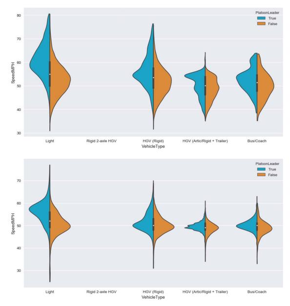
B.7 Speed profile for vehicles travelling in platoon vs "unconstrained" vehicles, Kincraig (Site JTC00355), from top to bottom: 2013 and 2015
