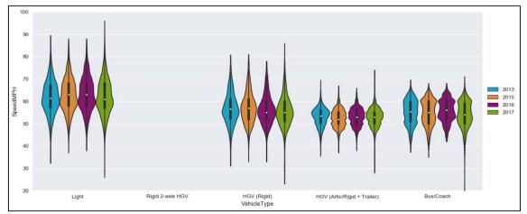
Figure 5-2 Change in vehicle speeds on dual carriageway section (violin plot)
