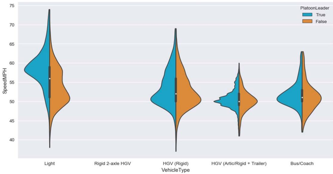
B.4 Speed profile for vehicles travelling in platoon vs “unconstrained” vehicles, Dalwhinnie (Site JTC00311), from top to bottom: 2013 and 2015
