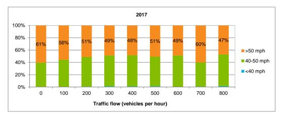
Based on available data, improved HGV speed limit compliance extended to the dual carriageway section where speed limits remained unchanged and there are no ASCs. Improvements in compliance amounted to around 14pp, between 2013 and 2015, and applied to both HGVs (>7.5 tonnes) which were subject to the limit change on single carriageway sections, and HGVs in the rigid (mixed weight) classes where applicability of the change was mixed.
