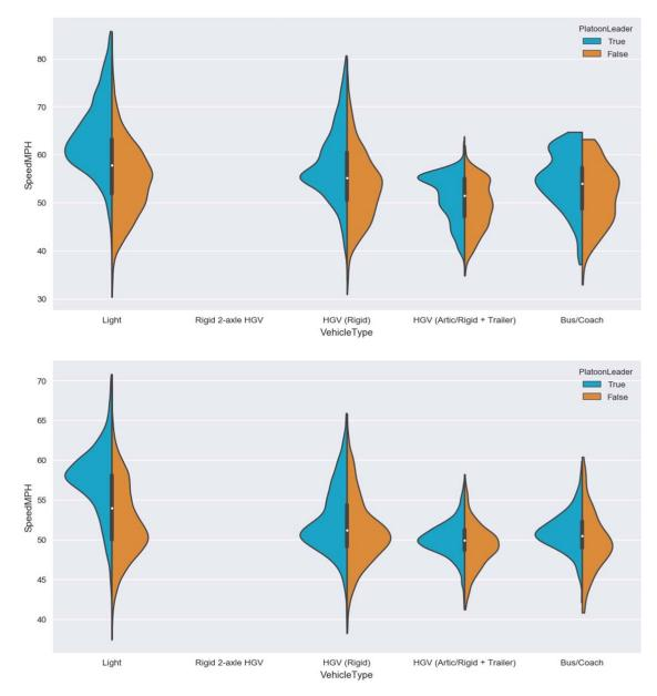
B.5 Speed profile for vehicles travelling in platoon vs "unconstrained" vehicles, Ralia (Site JTC00352), from top to bottom: 2013 and 2015
