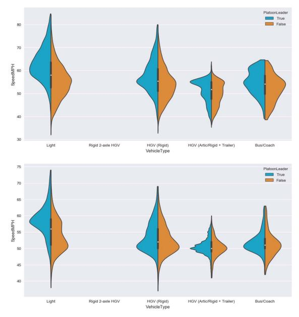
B.4 Speed profile for vehicles travelling in platoon vs "unconstrained" vehicles, Dalwhinnie (Site JTC00311), from top to bottom: 2013 and 2015
