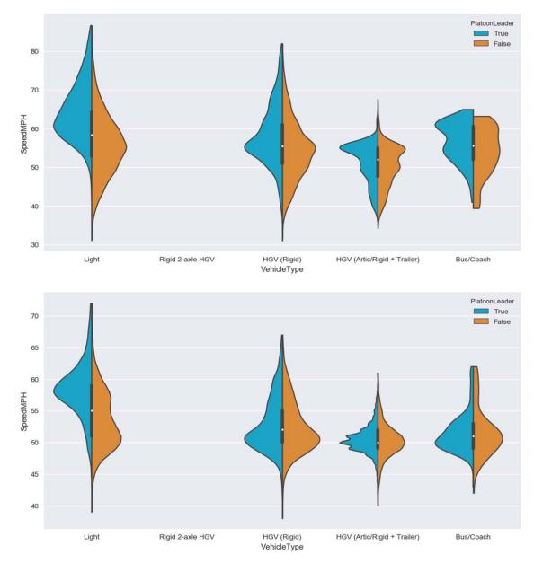
B.8 Speed profile for vehicles travelling in platoon vs "unconstrained" vehicles, Moy (Site JTC00368), from top to bottom: 2013 and 2015
