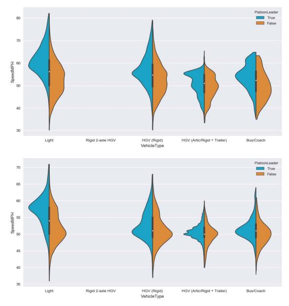
B.2 Speed profile for vehicles travelling in platoon vs "unconstrained" vehicles, Calvin (Site JTC00308), from top to bottom: 2013 and 2015
