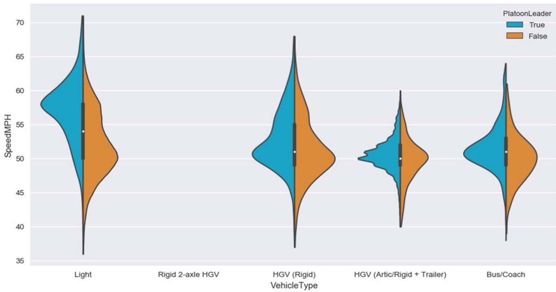
B.2 Speed profile for vehicles travelling in platoon vs “unconstrained” vehicles, Calvin (Site JTC00308), from top to bottom: 2013 and 2015
