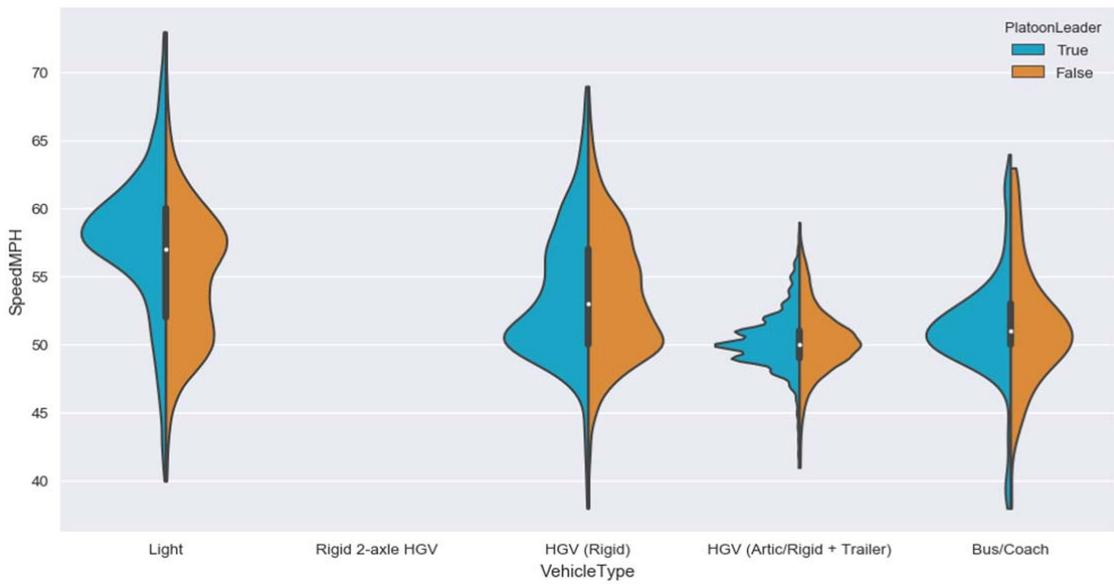
B.6 Speed profile for vehicles travelling in platoon vs "unconstrained" vehicles, Kingussie (Site JTC00312), from top to bottom: 2013 and 2015
