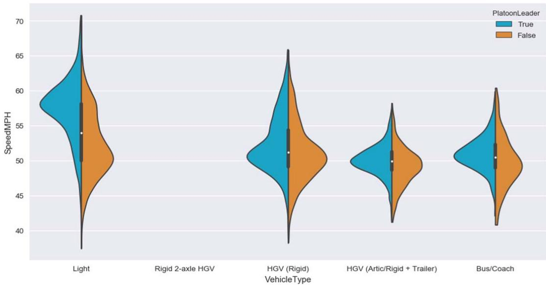
B.5 Speed profile for vehicles travelling in platoon vs “unconstrained” vehicles, Ralia (Site JTC00352), from top to bottom: 2013 and 2015
