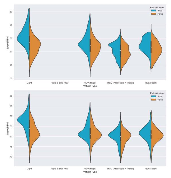
B.3 Speed profile for vehicles travelling in platoon vs "unconstrained" vehicles, Dalnaspidal (Site JTC00310), from top to bottom: 2013 and 2015
