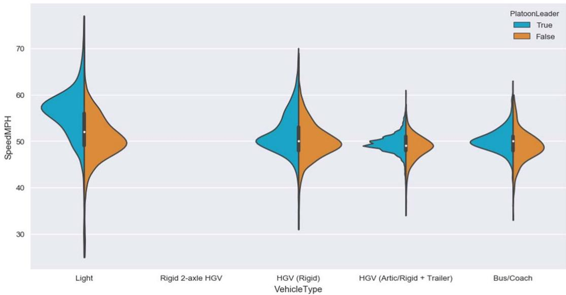
B.7 Speed profile for vehicles travelling in platoon vs “unconstrained” vehicles, KinCraig (Site JTC00355), from top to bottom: 2013 and 2015
