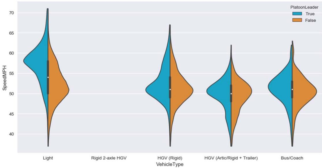
B.3 Speed profile for vehicles travelling in platoon vs “unconstrained” vehicles, Dalnaspidal (Site JTC00310), from top to bottom: 2013 and 2015
