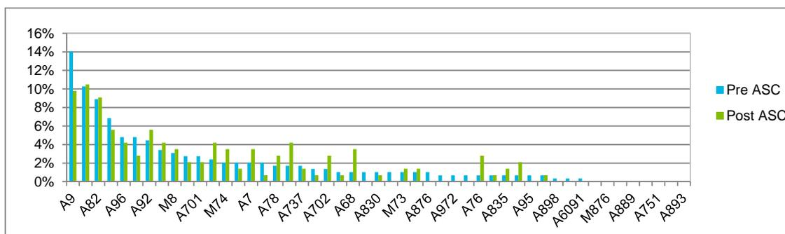
**Figure 7-1 Proportion of fatal accidents by road, Impact of the ASC implementation and HGV speed limit reduction**
