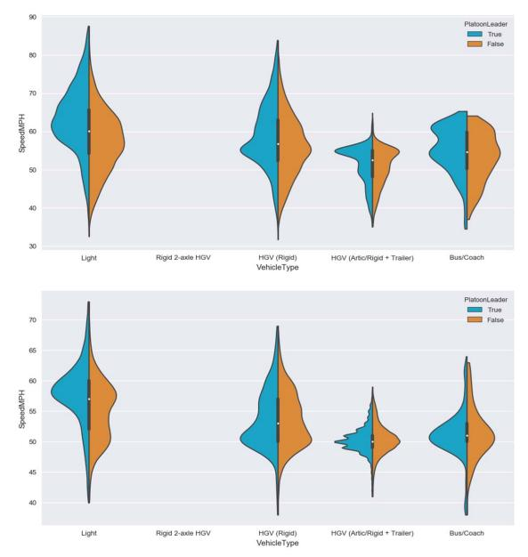
B.6 Speed profile for vehicles travelling in platoon vs "unconstrained" vehicles, Kingussie (Site JTC00312), from top to bottom: 2013 and 2015
