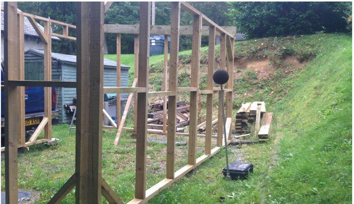
2.1.2 The monitoring equipment was calibrated both before and after the measurement period using an Rion NC-74 (s/n 34536108) acoustic calibrator, which has itself been calibrated against a reference set traceable to National and International Standards. There was no significant shift in the observed calibration level.
