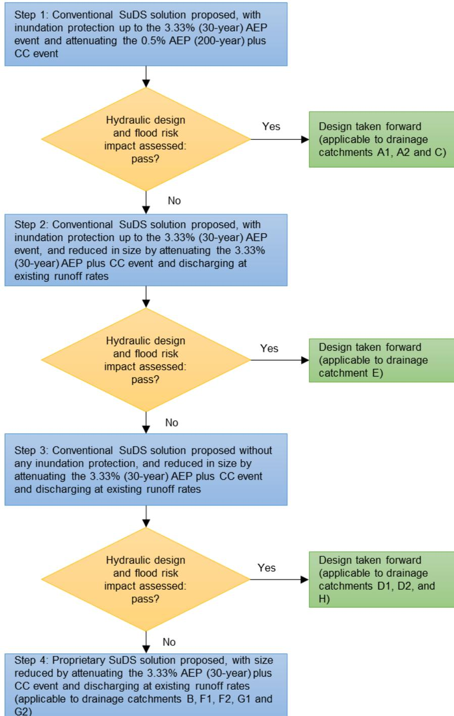
SuDS Departure 1: Maintaining Existing Discharge Rates & 3.33% AEP Attenuation Volume
