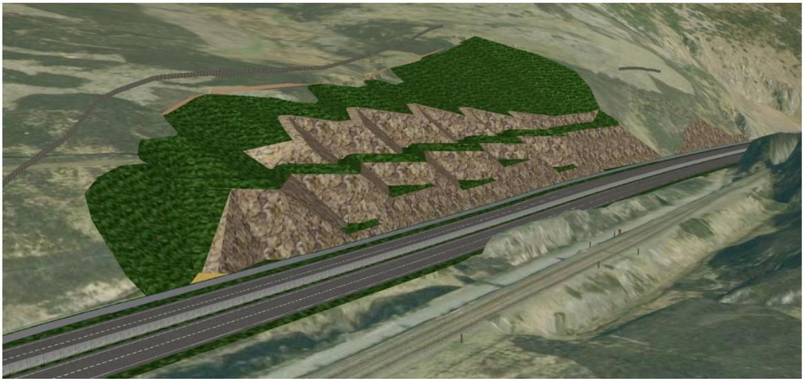
**Figure 4.1: 3D Model of Rock Cut Design at Slochd Summit**
