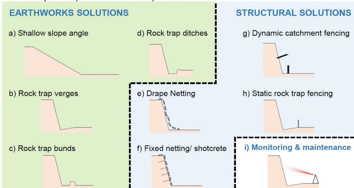
Figure 1.1: Overview of Principles Considered for each Proposed Rock Cut
