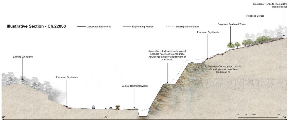
Figure 4.9: Illustrative Section at Ch.22000 showing Proposed Rock Cut at Slochd Beag
