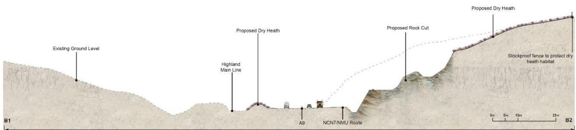
**Figure 4.3: Illustrative Section at Ch.24000 showing Proposed Rock Cut at Slochd Summit**
