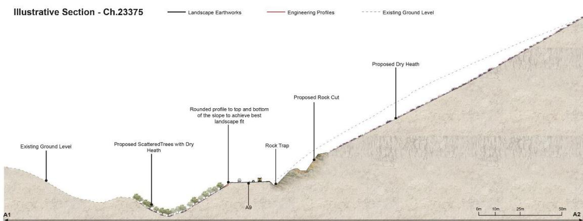
**Figure 4.6: Illustrative Section at Ch.23375 showing Proposed Rock Cut at Slochd Mor**
