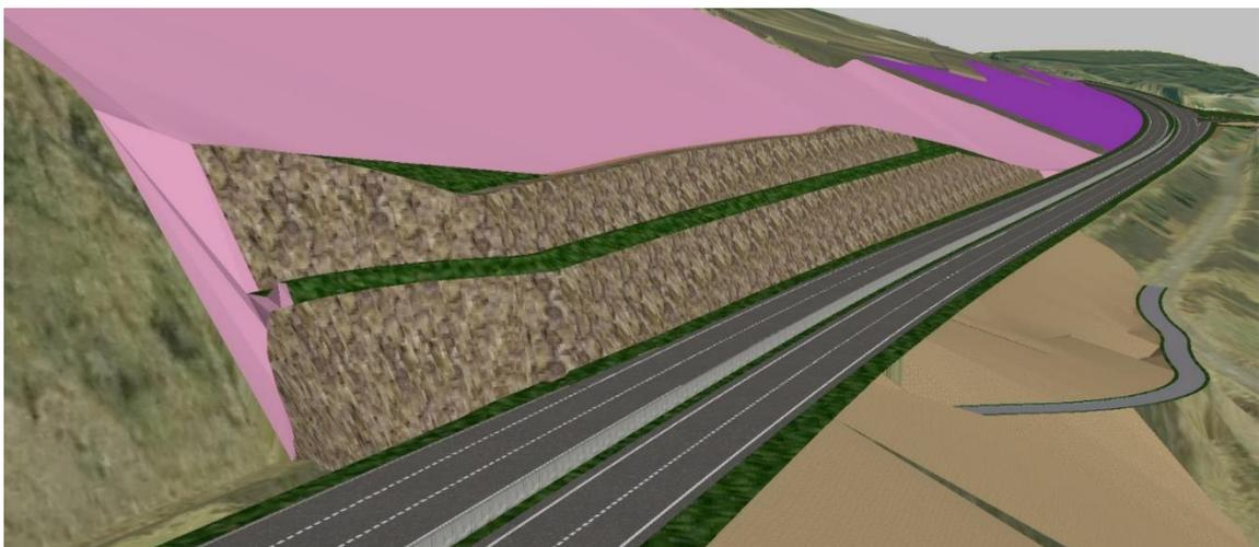
**Figure 4.5: 3D Model of Rock Cut Design at Slochd Mor**
