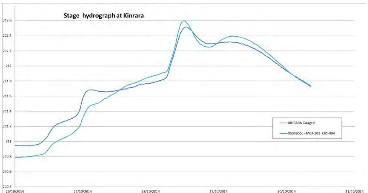
*Figure B2-2: October 2014 – Stage hydrograph at Kinrara gauging station*
