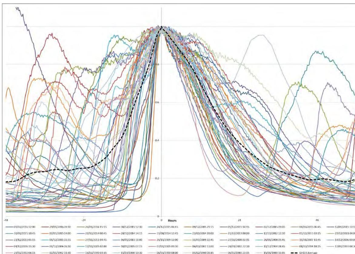
Figure A5-2: Standardised synthesised hydrograph for 8007 River Spey @ Invertrium
