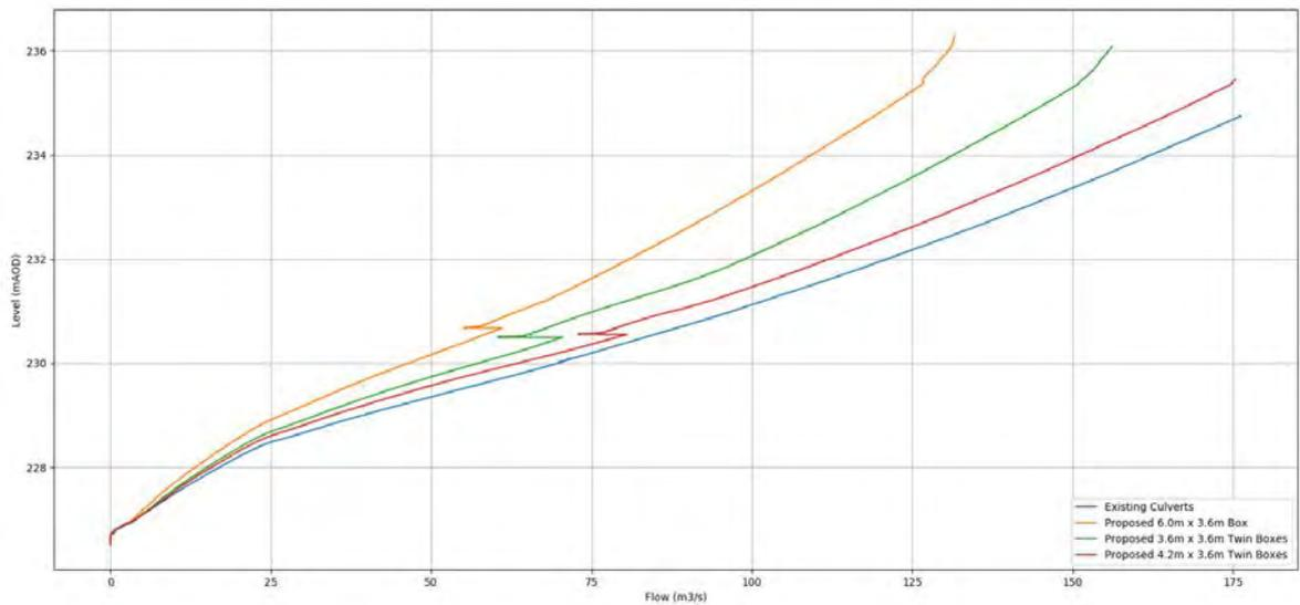
Figure B6-1: ID147 and downstream access track – Upstream flood level as a function of the flow downstream of the access track, Existing conditions and four proposed A9 crossing arrangements.
