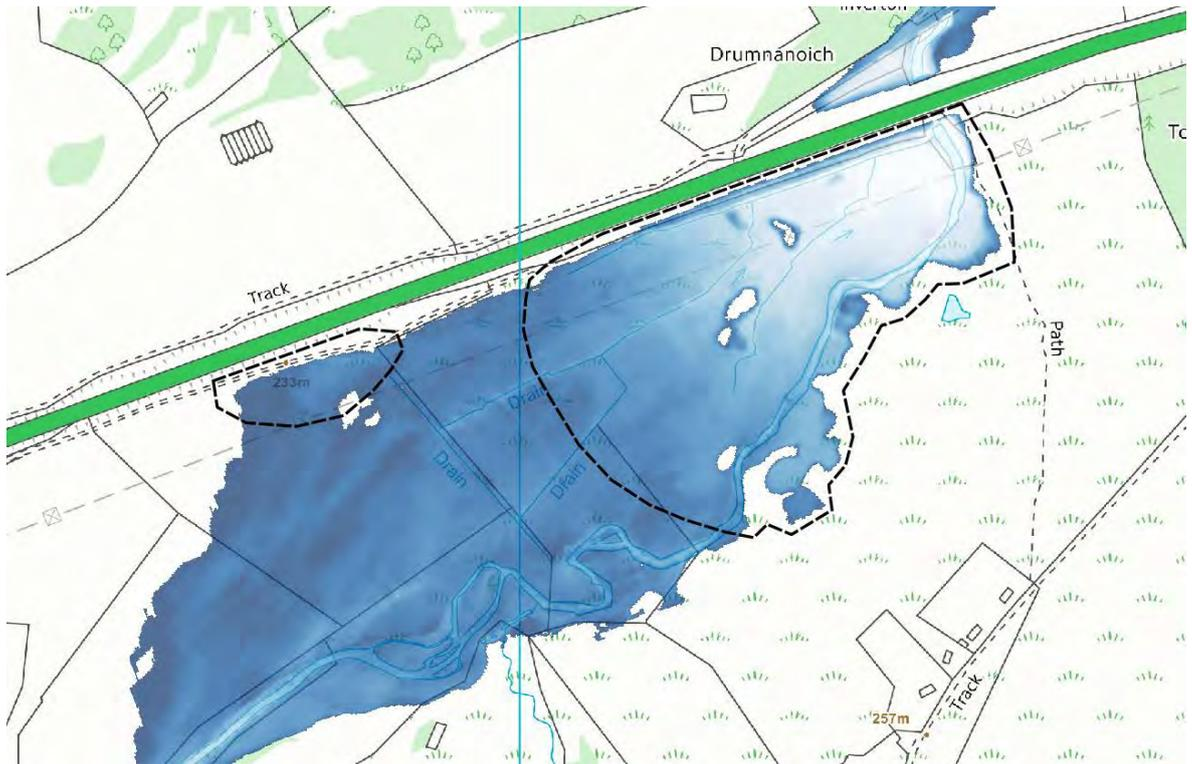
Figure B6-2: ID147 Flood extent and upstream areas where there is a noticeable difference in flood levels between extending and proposed conditions (existing depths shown).
