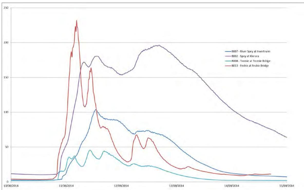
Figure B2-4: August 2014 – Flow hydrographs at gauging stations
