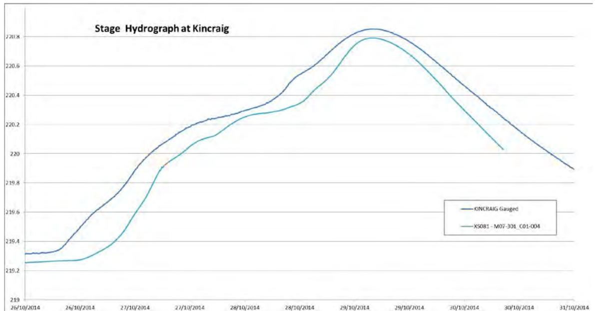
Figure B2-3: October 2014 – Stage hydrograph at Kincaig level station
