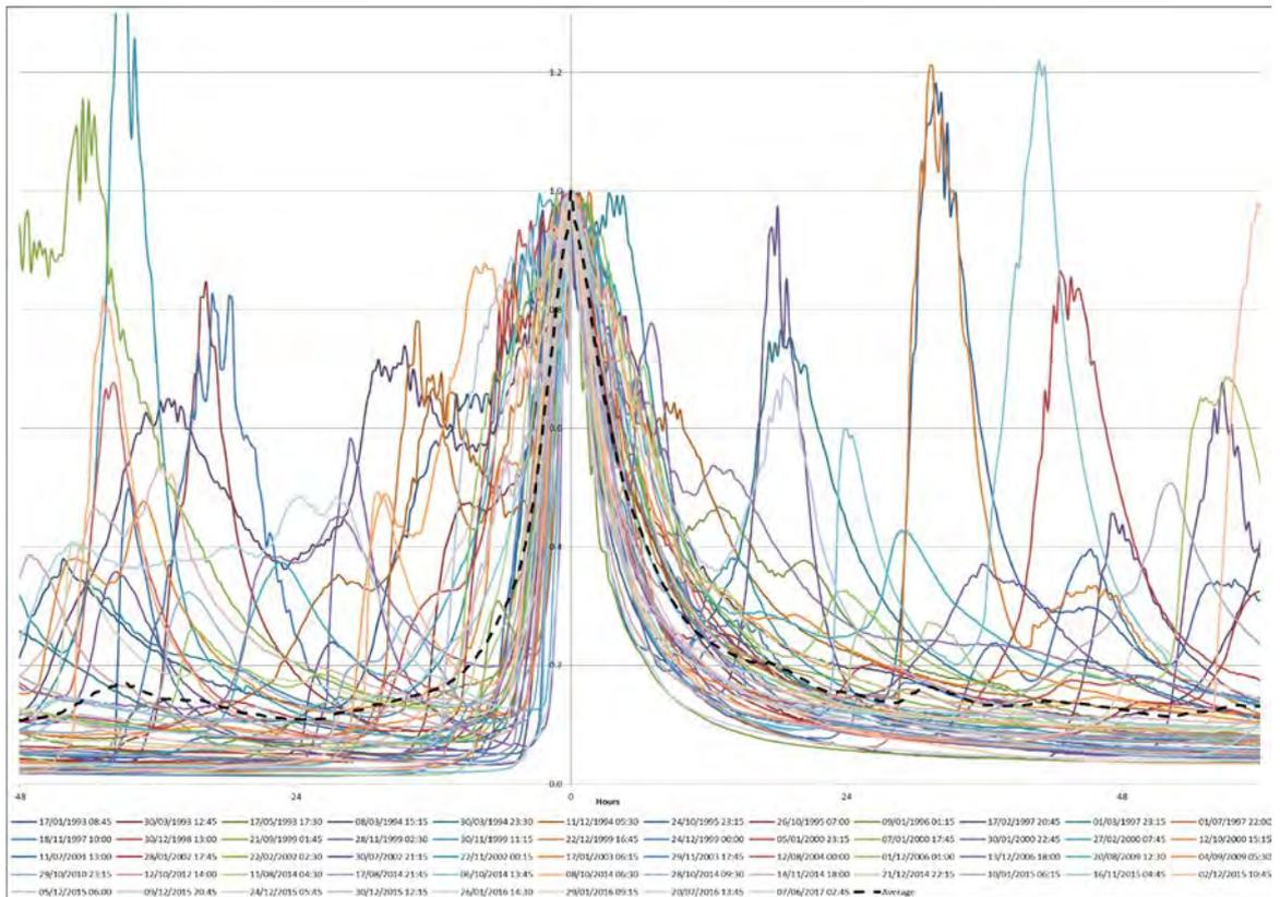
Figure A6-2: Standardised synthesised hydrograph for 8013 River Feshie @ Feshie Bridge
