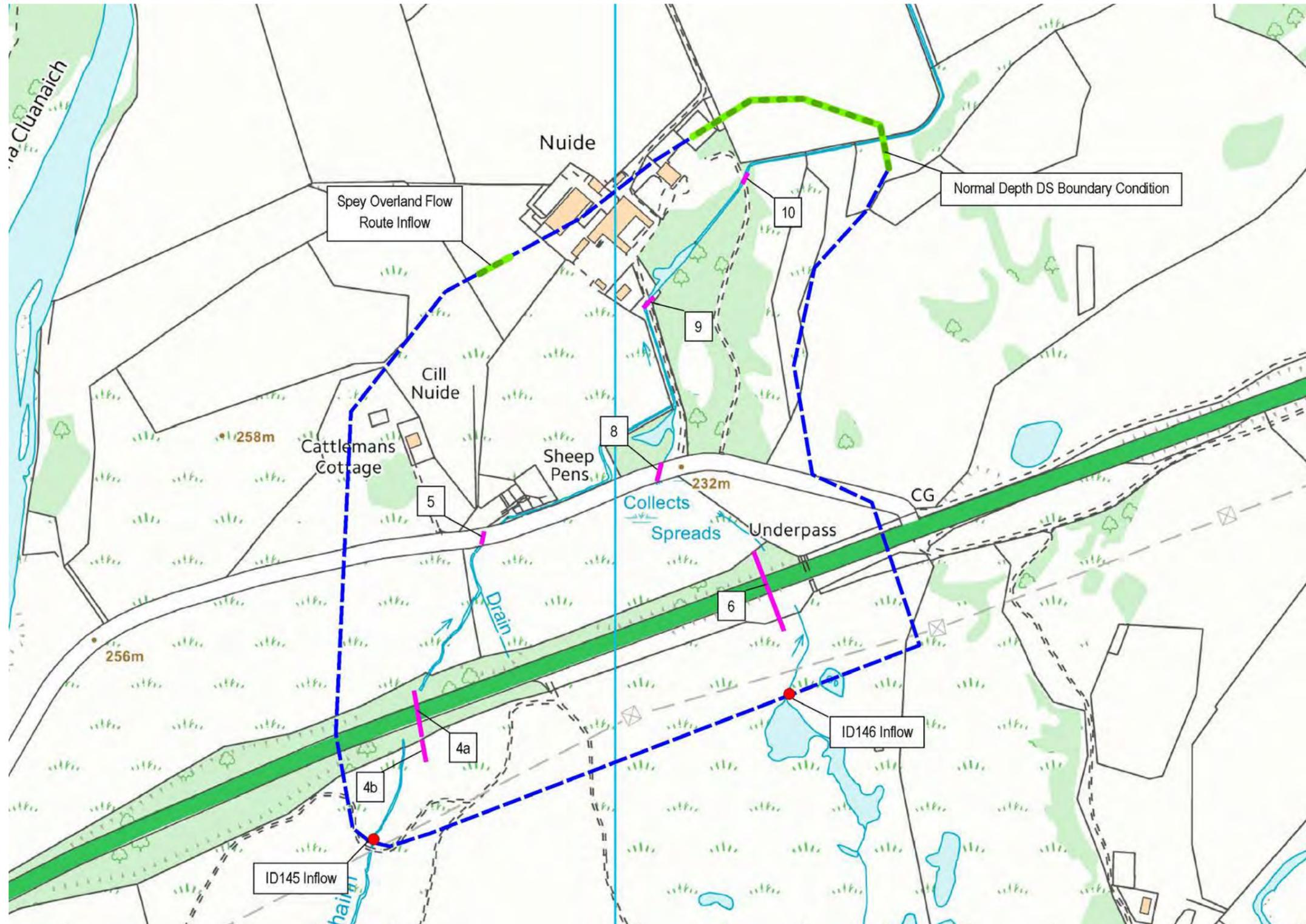
Figure B5-6: Proposed Model Layout, ID145 and ID146
