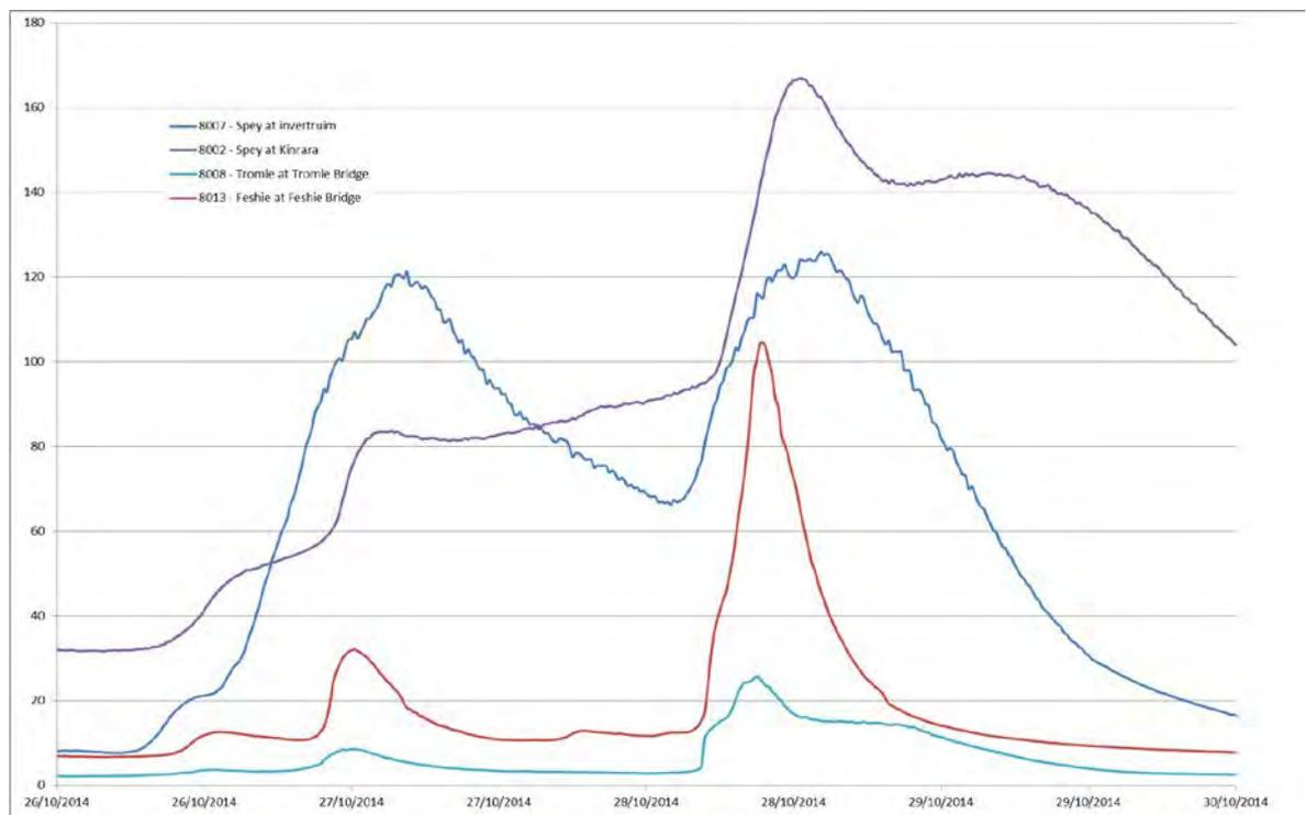
Figure B2-1: October 2014 - Flow hydrographs at gauging stations
