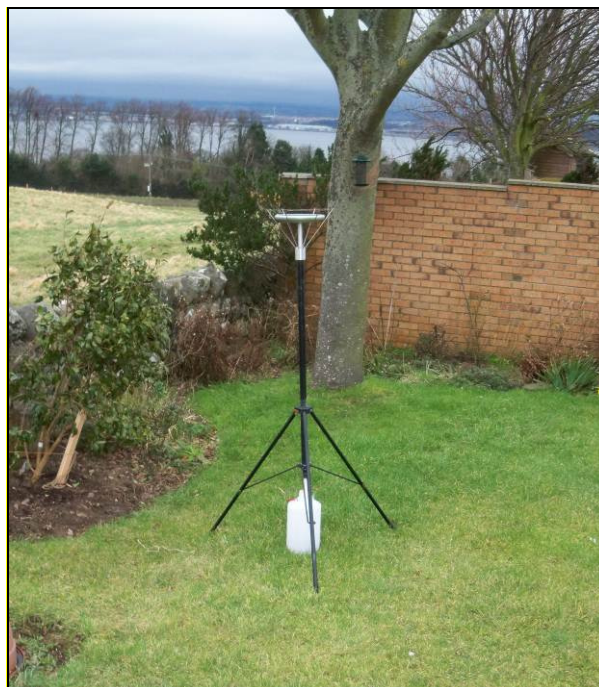
Figure 1: Example of an Installed Frisbee Gauge Meter
