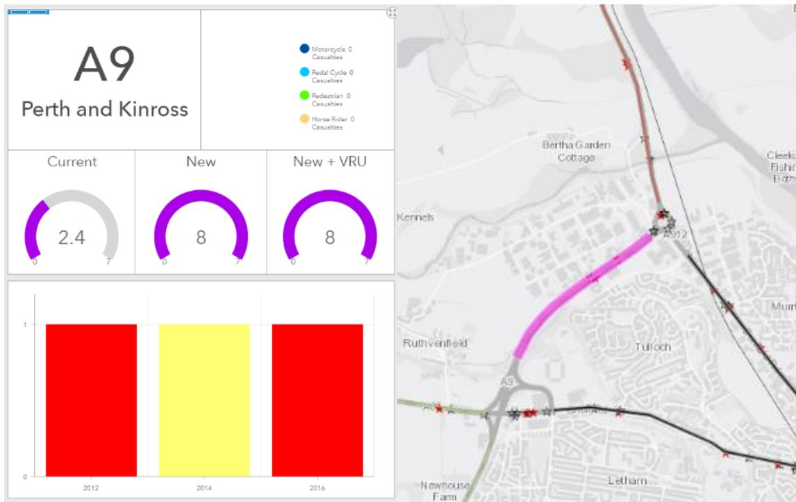
The A9 between the A85 and A912 on the north-west of Perth was also not eligible for consideration under the *current* criteria. The 1.25km from the roundabout towards the south-west is where the collisions occurred and could be considered for a fixed camera site. There were 2 serious and 1 slight casualties over the five years, amounting to total points of 10 and a rate of 8.77 points per km, meeting the *new* criteria.
