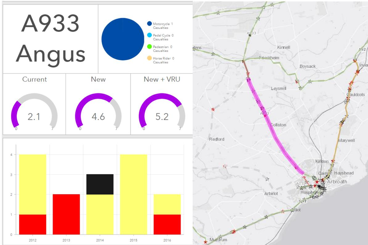
The A933 from Arbroath north-west, past Colliston, towards Forfar would not be considered as a site under the *current* criterion. Using either of the proposed systems, the entire route of 7.6km would also not meet the *new* criteria.
