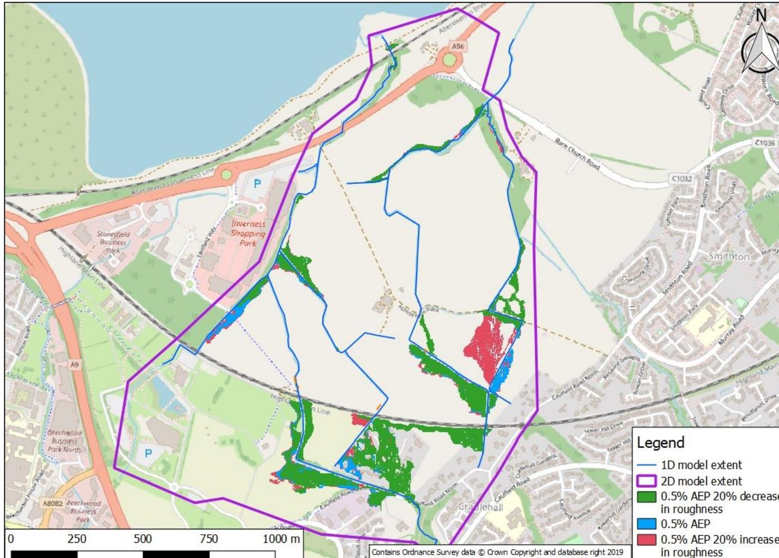
**Figure 16: Inflow sensitivity 2D flood modelled flood extents**
