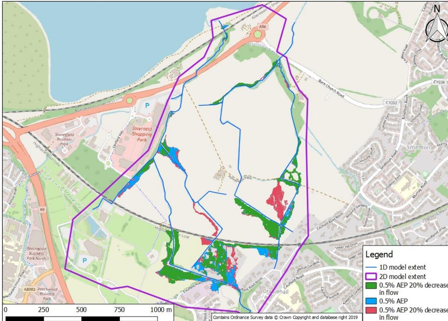
**Figure 17: Downstream Boundary sensitivity 2D flood modelled flood extents**
