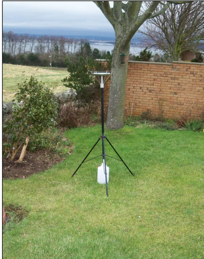
**Figure 1: Example of an Installed Frisbee Gauge Meters**
