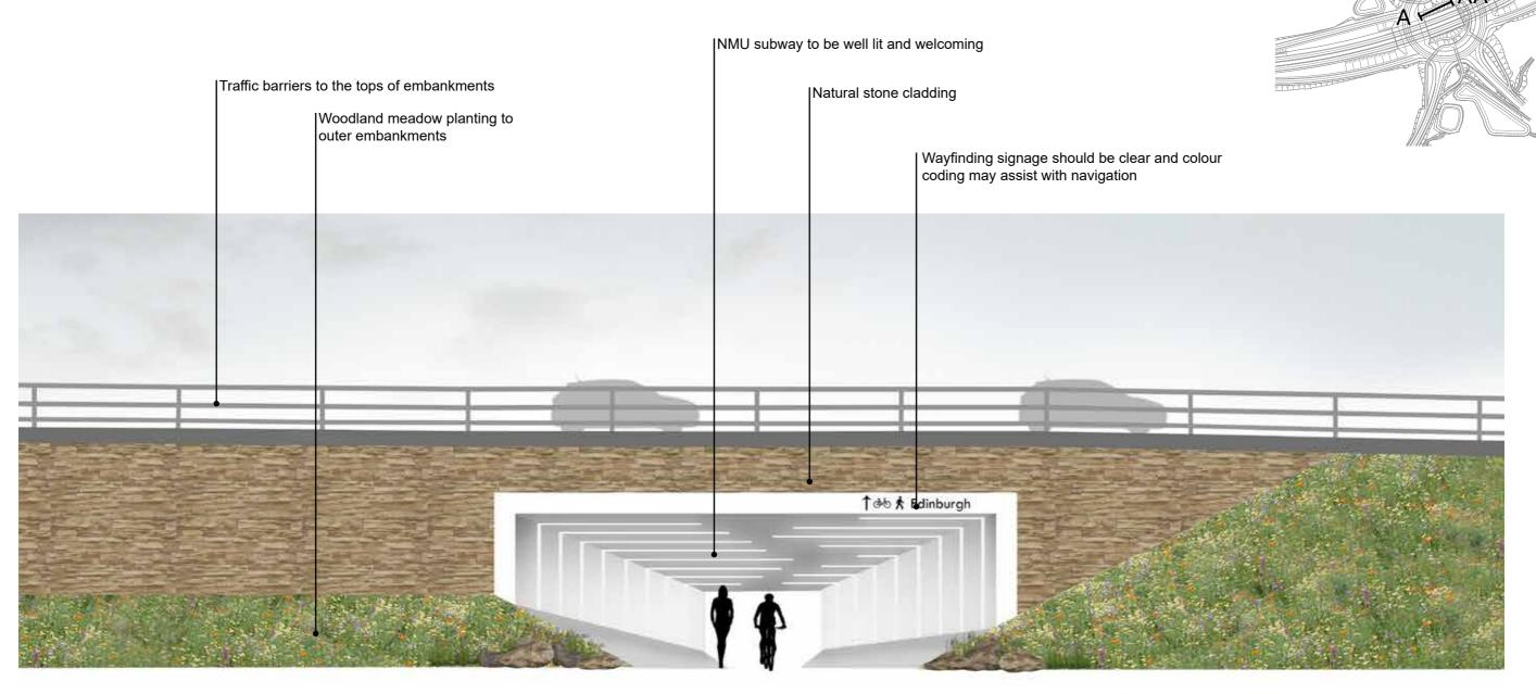
Elevation A:AA - Elevation through roundabout looking north towards NMU Entrance (NTS)
