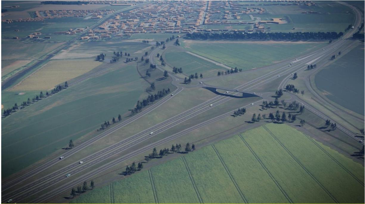
The A90/A937 Laurencekirk Junction Improvement Scheme comprises a new grade-separated junction located at the existing at-grade south junction into Laurencekirk from the A90. The scheme design is shown in **NTS Figure 1**.
