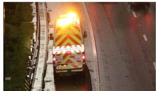
**A TRISS vehicle with an illuminated vehicle panel**
