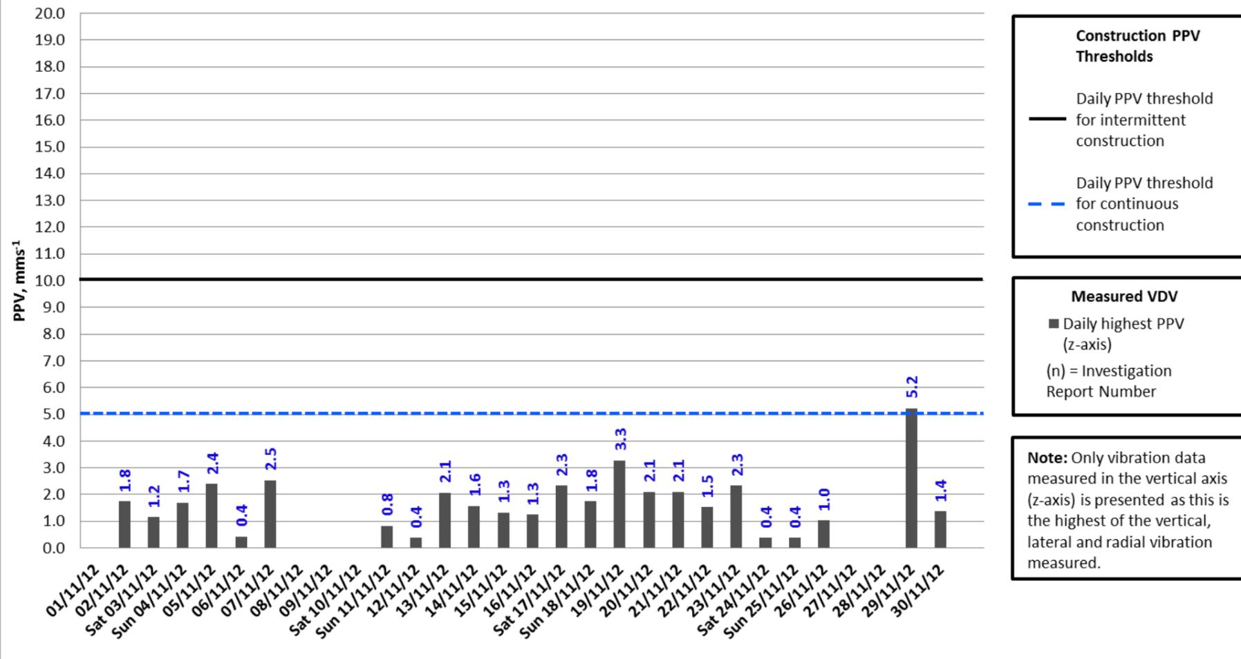
**Construction PPV Thresholds**
