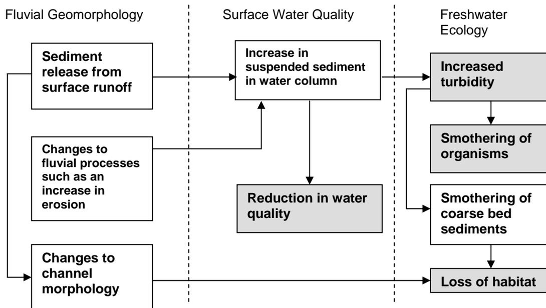
**Figure 1 – Conceptual diagram illustrating the relationships between impacts on fluvial geomorphology, water quality and ecology (grey denotes an impact on receptor)**
