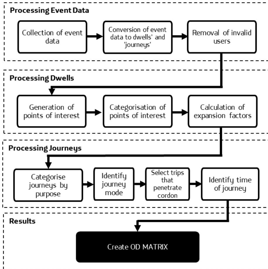
Figure 3: Process diagram of the existing methodology.
