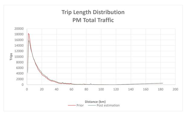
Figure 24. PM Trip Length Distribution for Prior and Post-Matrix Estimation
