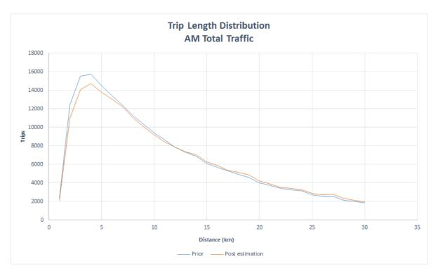
Figure 25. AM Trip Length Distribution for Prior and Post-Matrix Estimation (<30km)
