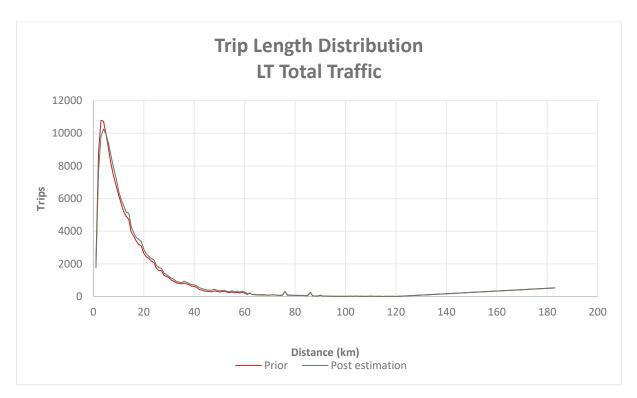
Figure 23. LT Trip Length Distribution for Prior and Post-Matrix Estimation
