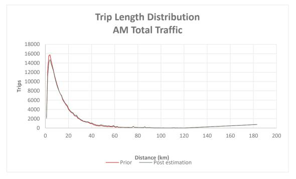
Figure 22. AM Trip Length Distribution for Prior and Post-Matrix Estimation
