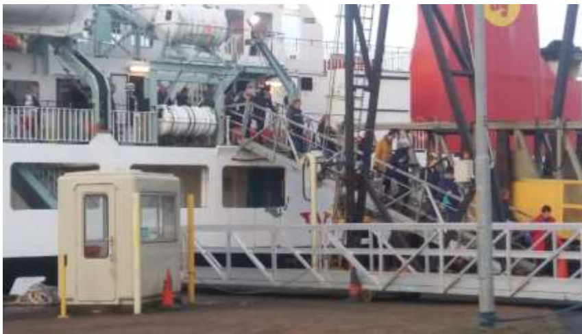
Photo 1. The gangway at Ardrossan showing a 45 0 angle, which is extremely difficult for disabled travellers to negotiate.
