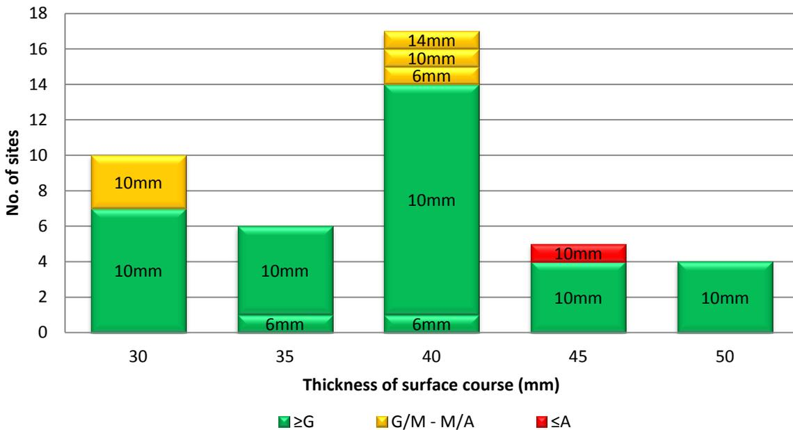
Figure 4.8: TS2010 layer thickness versus performance
