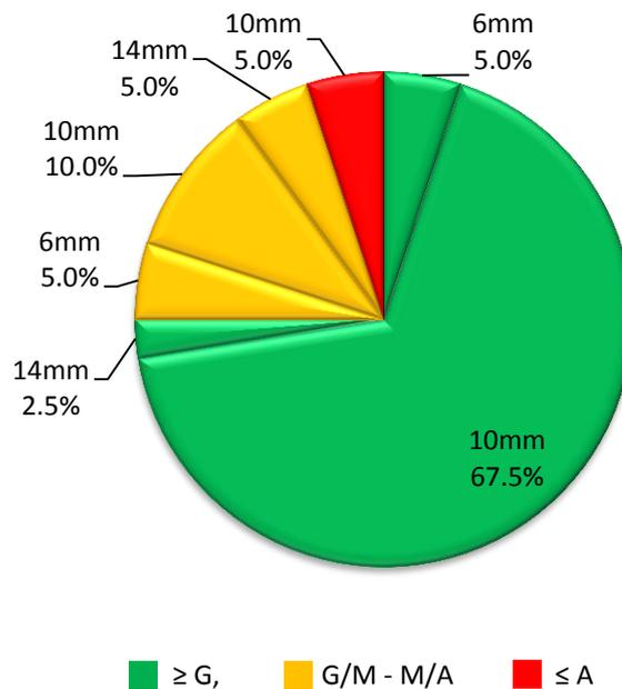
Figure 4.1: Aggregate size used for two-year-old sites
