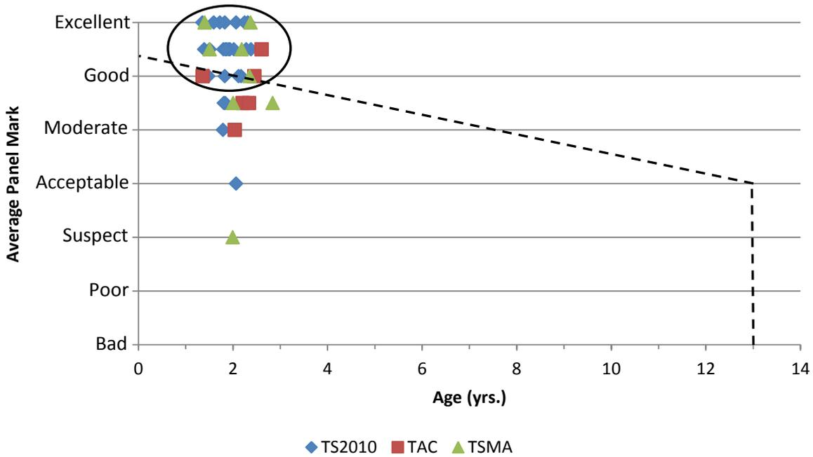
**Figure 3.2: Average condition markings versus performance**
