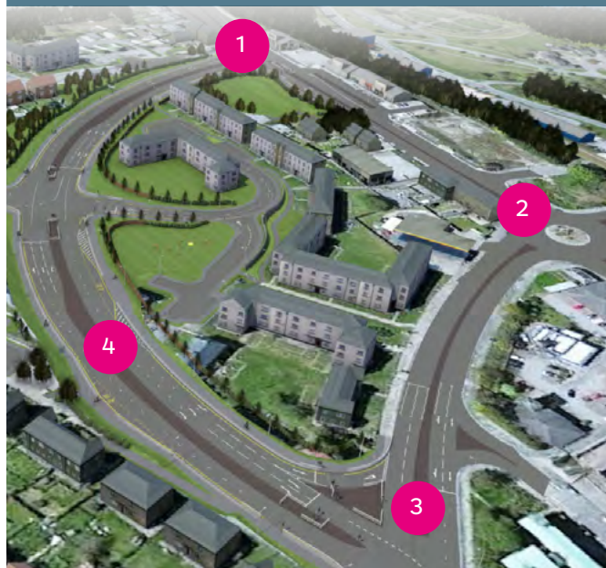
Contraflow traffic management on the A96, allowing works to progress to connect the new link road junction, retaining wall and works on drainage basin to continue
