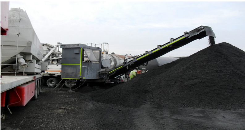
Figure 2: Mobile treatment of Waste Tar Bound Planings (photo courtesy of A-one+)
