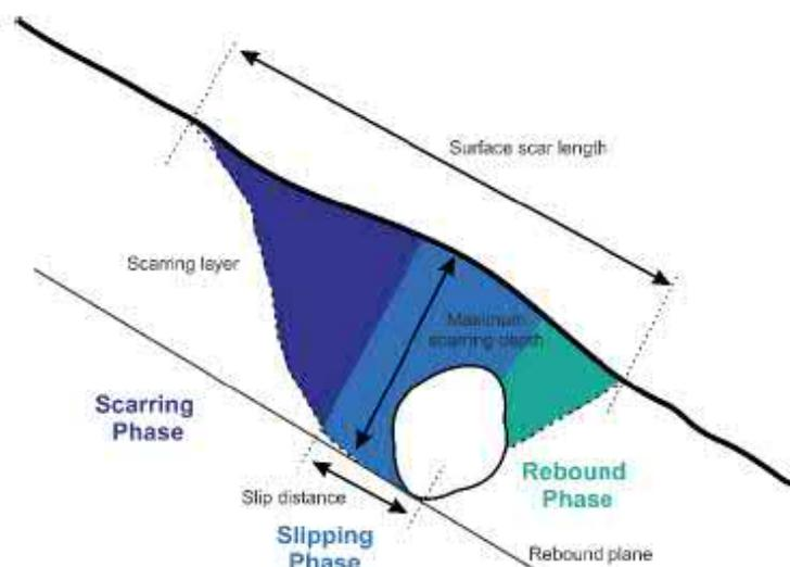
Figure 6-1: Illustration of the three distinct phases of rock-terrain interaction implemented in RAMMS: Rockfall – scarring phase, slipping phase, and rebound phase (Caviezel et al., 2019).
