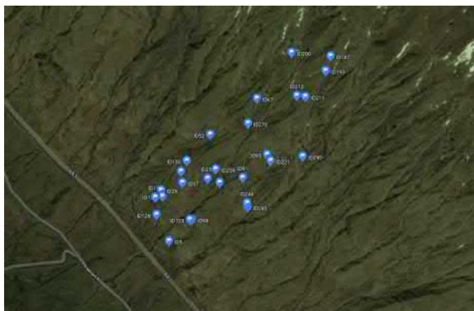
Figure 6-7: Release points of boulders selected for detailed simulation
