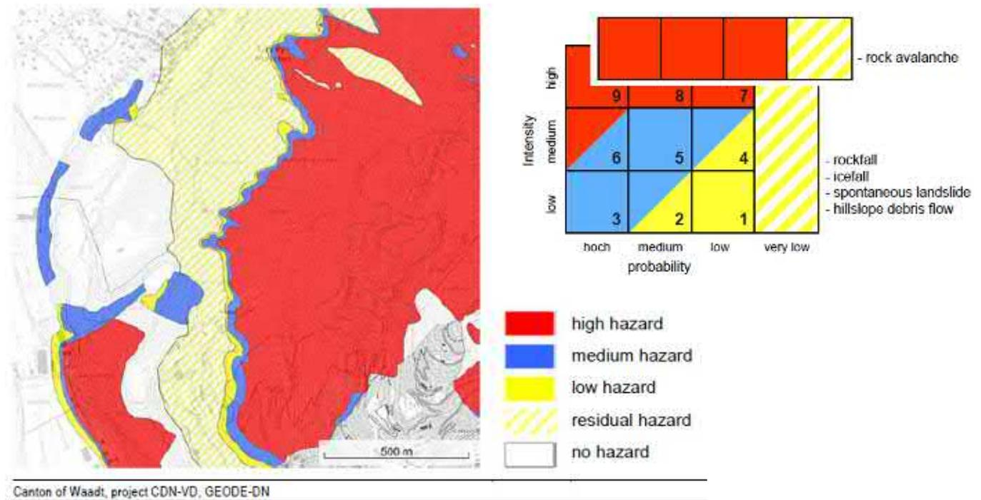
Figure 3.3 – Magnitude-probability diagram and example of rockfall hazard map from Canton of Waadt, (Raetzo and Loup, 2016).
