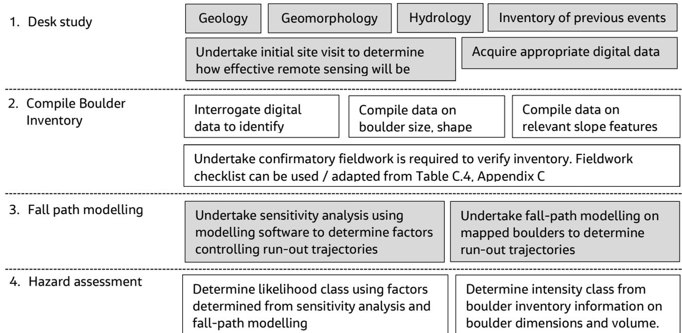
**Figure 8-1:** Outline methodology for determining boulder hazards
