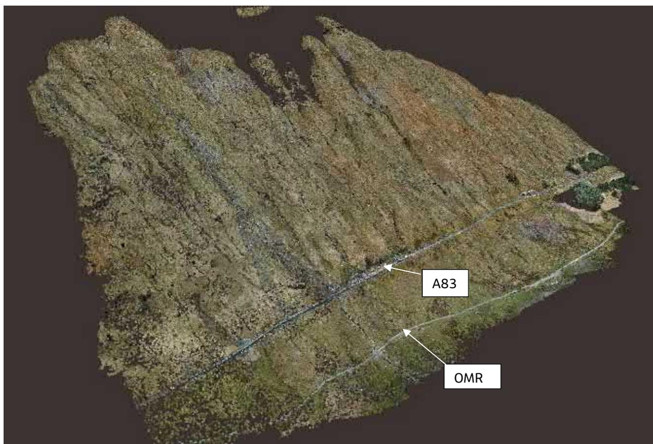
Figure 4-2 - DEM prepared using UAV photogrammetry
