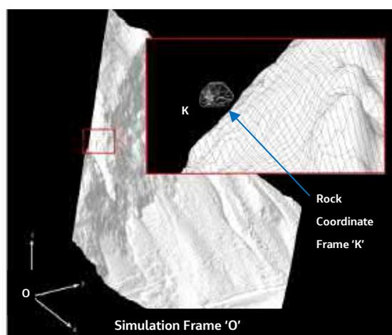
Figure 6-2: Simulation frame O, comprising a tessellated terrain surface with which rock bodies (K) can come into contact (Bartelt et al., 2016).
