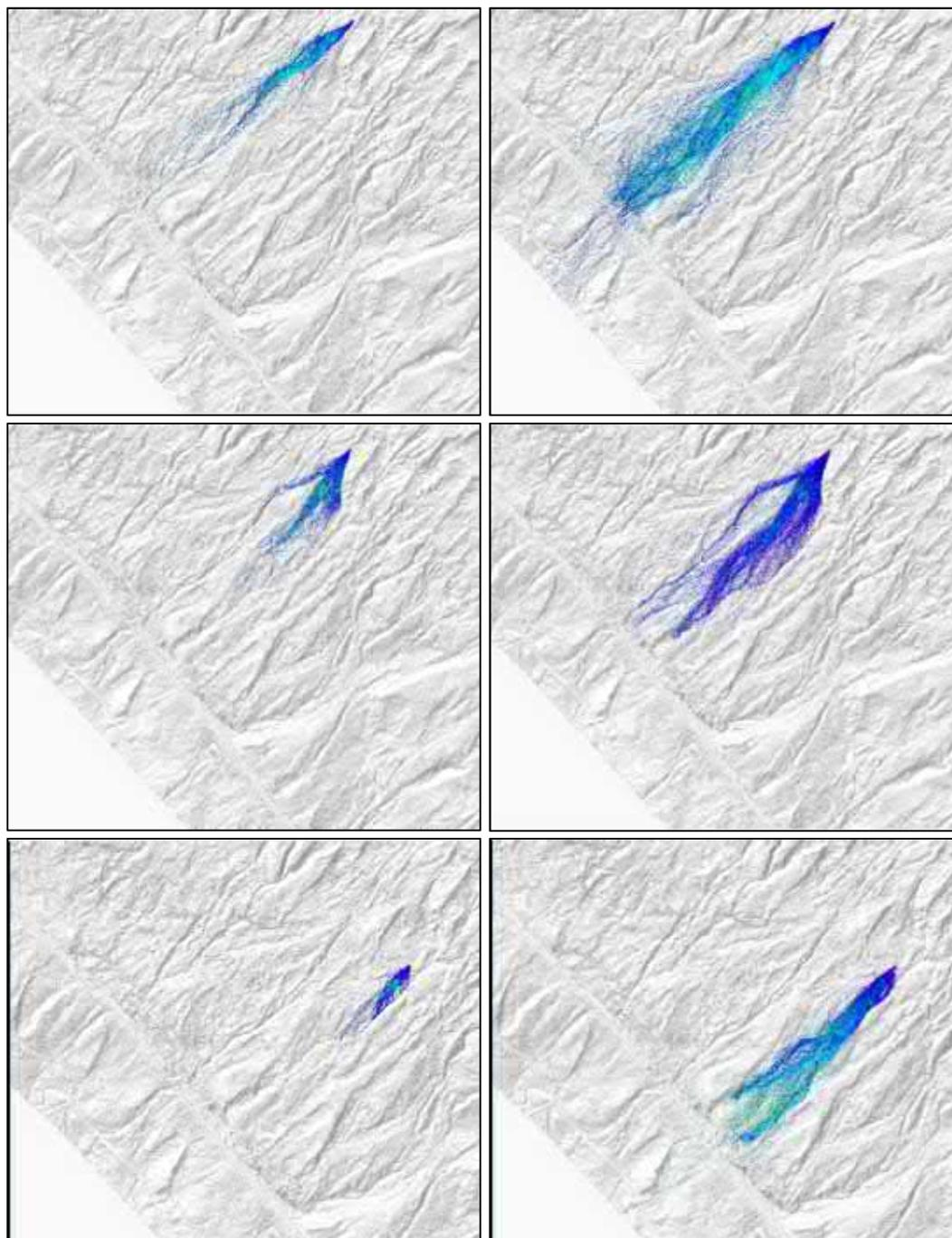
Figure 6-8: Comparison of runout trajectories of long (left) and equant (right) shape boulders with the same volume, mass and starting position characteristics.
