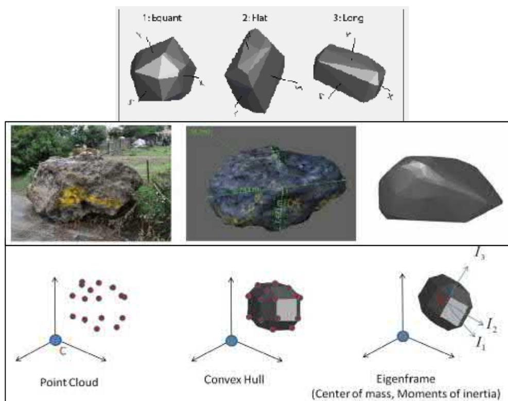
Figure 6-3: Equant, flat and long convex-hull polyhedrons that represent real boulders have been built using point clouds of Swiss boulders. These pre-built boulders can be used for modelling. Site-specific rock libraries can also be compiled if unique boulder point clouds are available (Bartelt et al., 2016).
