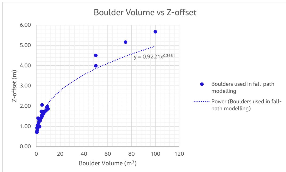
Figure 7-1: Power law relationship between boulder volume and Z-offset. In this functional relationship, a relative change in boulder volume results in a proportional relative change in Z-offset.
