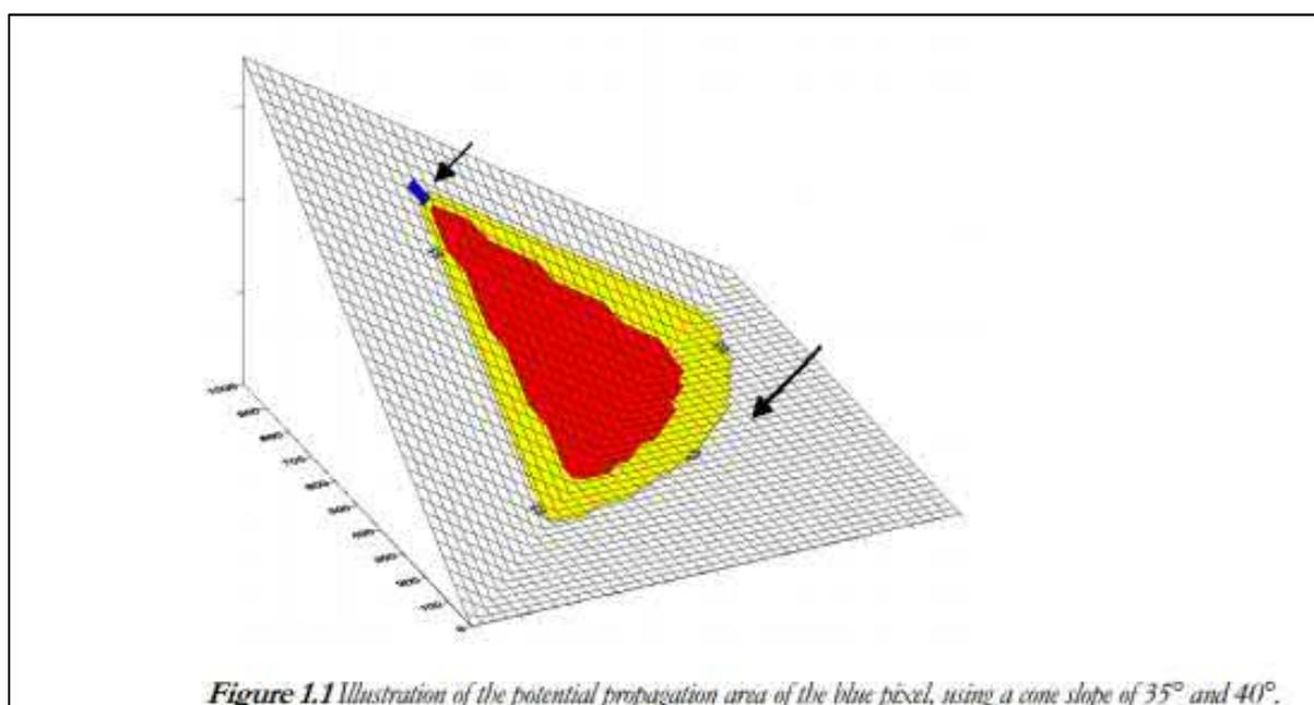
Figure 3-3 – Model illustrating potential propagation of a boulder in CONEFALL for a defined slope angle. Taken from program user manual (Jaboyadoff 2003).
