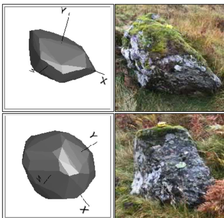
Figure 6-5: Boulders with a cuboid-like appearance were modelled using the long rock shape classification (top). Boulders with a shape that could be more closely approximated to a cube or a sphere (rather than a cuboid or cylinder) were modelled using the equant rock shape classification (bottom).
