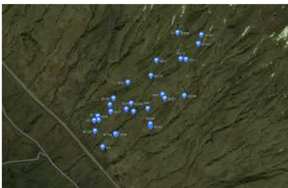
Figure 6-7: Release points of boulders selected for detailed simulation
