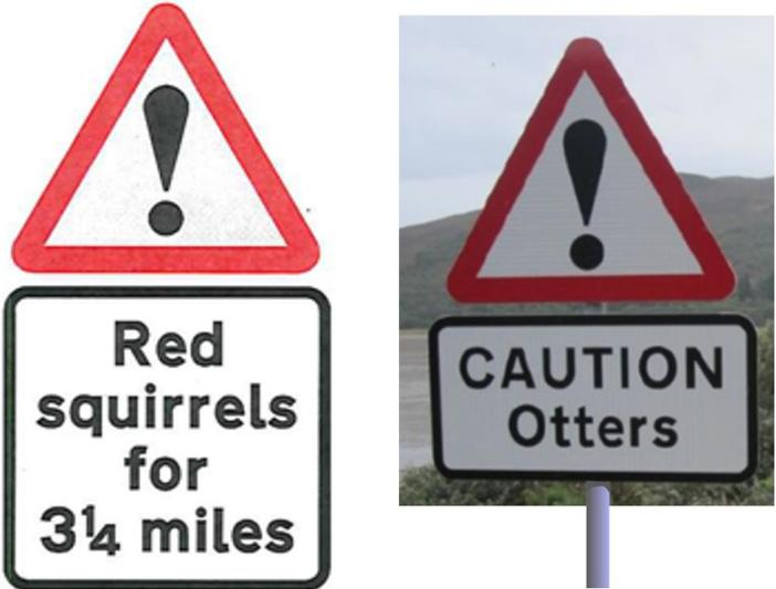
Figure 8 - Two examples of how the prescribed warning sign can be combined with additional plates to focus drivers’ attention on the possibility of encountering certain wildlife species in specific locations.
