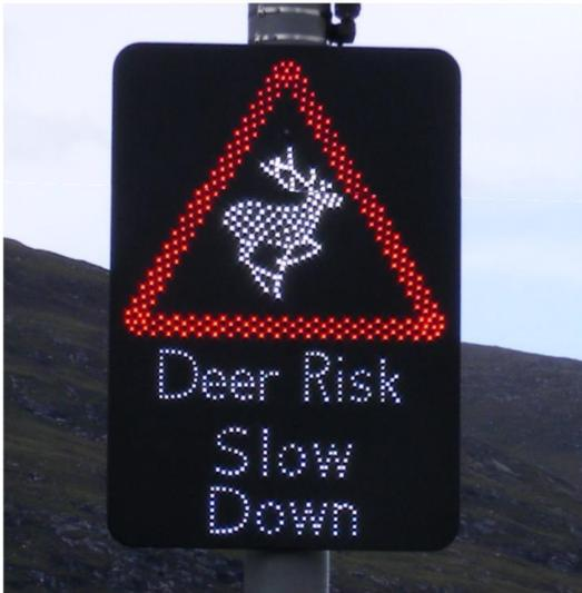
Figure 6 – Example of a speed-activated sign used in a trial on the Scottish trunk road network
