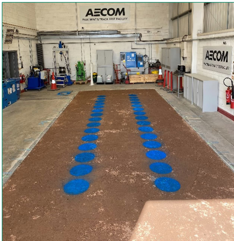
Figure 6 - Completed Test Pit with Test Locations
