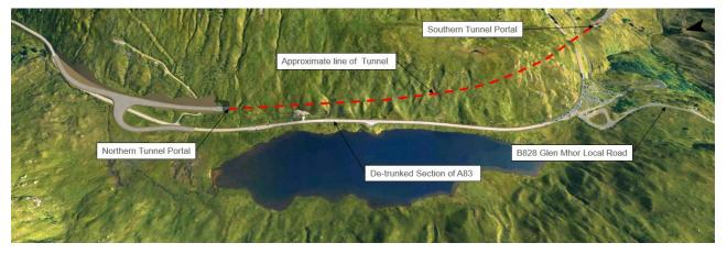
Figure 5-35 - Visualisation of the proposed B828 Glen Mhor local road junction with the Purple Option to the north-east of Loch Restil
