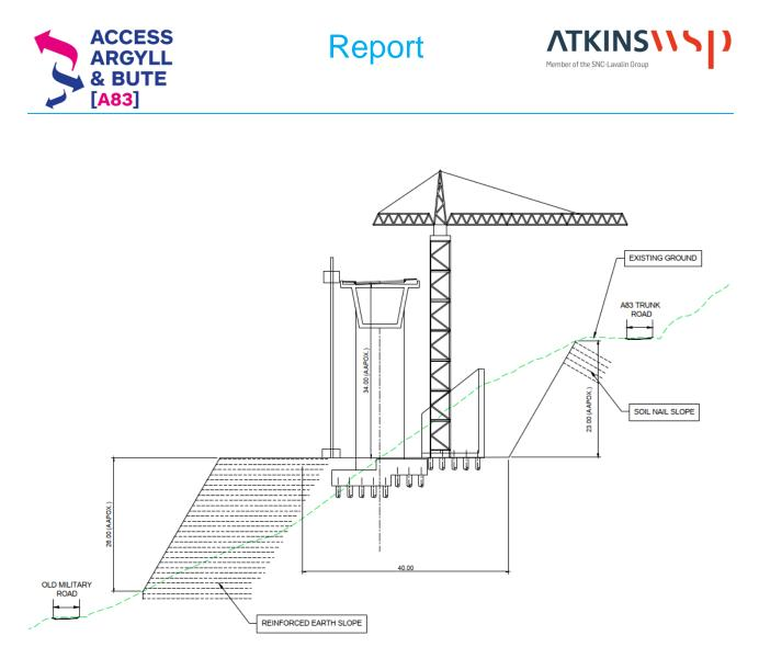
Figure 5-1 - Typical Temporary Works Footprint for Alignment Above OMR
