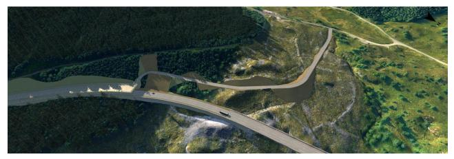
Figure 5-29 - Visualisation of the northern maintenance access from an existing forestry track that links to the B828 to the roof of the Green Option debris flow shelter
