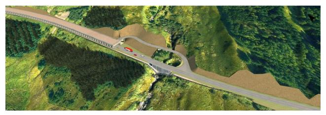
Figure 5-19 - Visualisation of the maintenance access to the roof of the Debris Flow Shelter for the Brown Option
