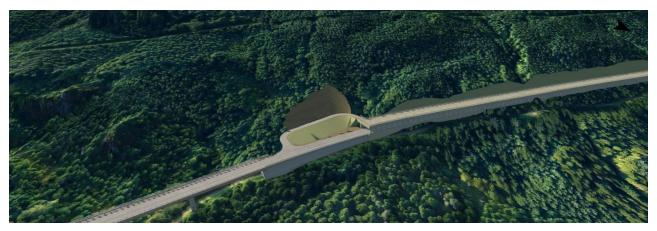
Figure 5-28 - Visualisation of the southern maintenance access from the proposed A83 to the roof of the Green Option debris flow shelter
