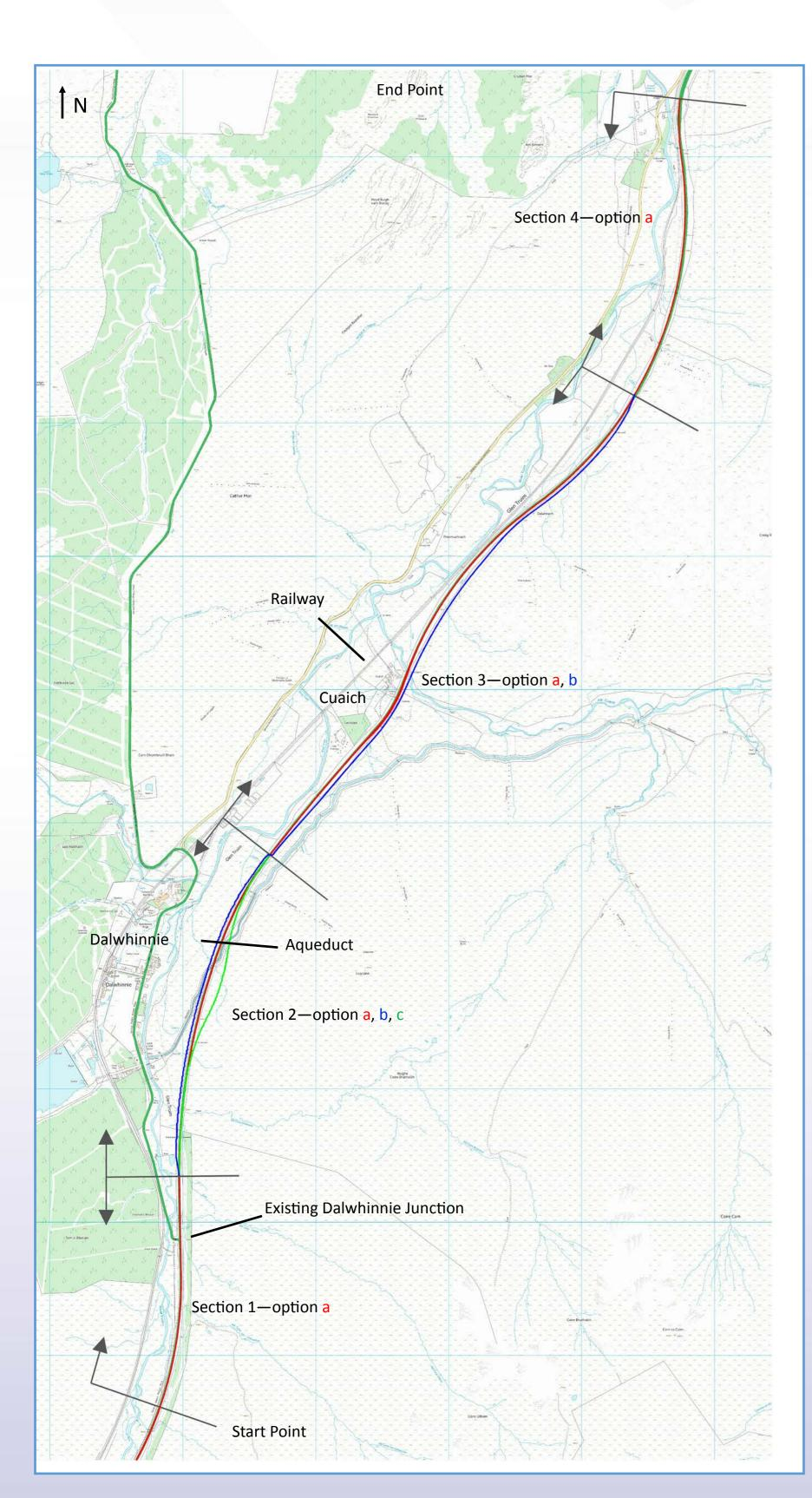
The project was split into four sections to aid design work on the dual carriageway options. The sections are shown on the adjacent map and were chosen based on adjacent constraints such as topography, environmental features and the proximity of the Highland Mainline railway.
