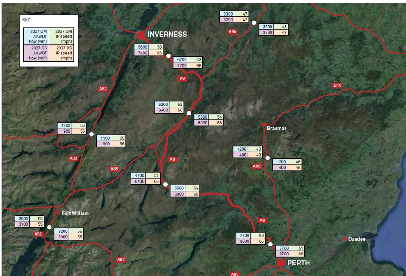
**Figure 5.1: Forecast Traffic Flows and Speeds with (DS) and without (DM) the A9 Dualling Programme (Excluding Average Speed Cameras)**
