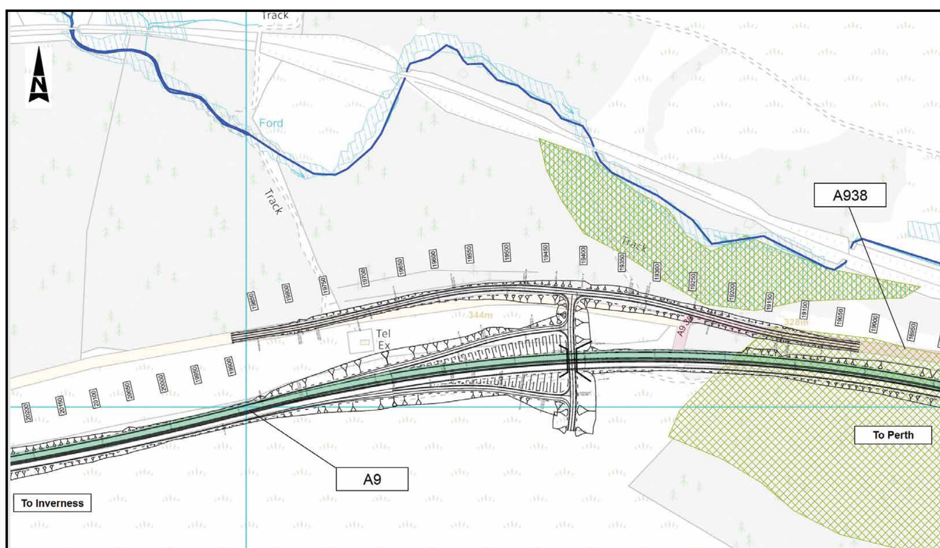
Half diamond (north-facing slips) layout developed to cater for the dominant north/south traffic movement between A9 and A938
