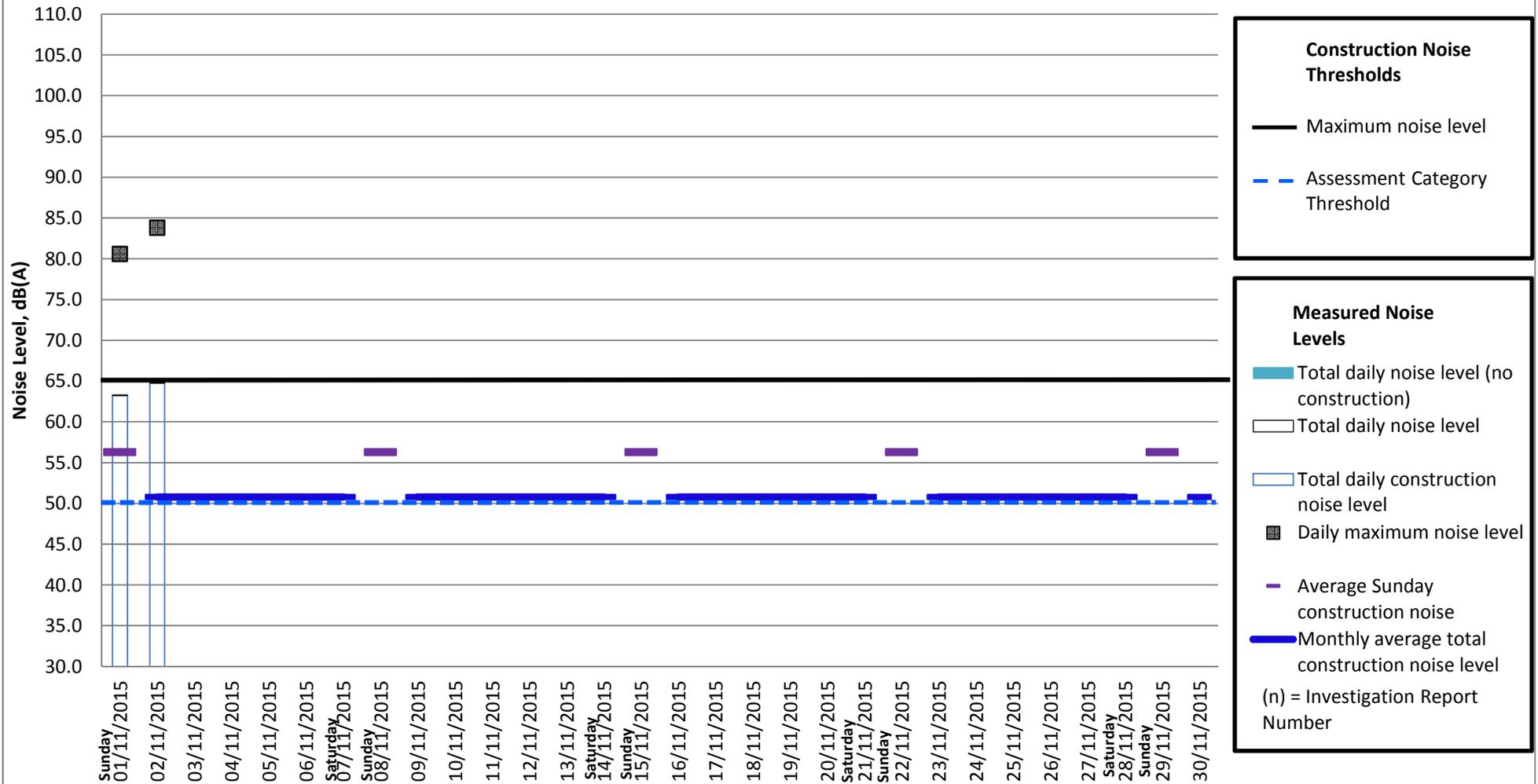
**Construction Noise Thresholds**
