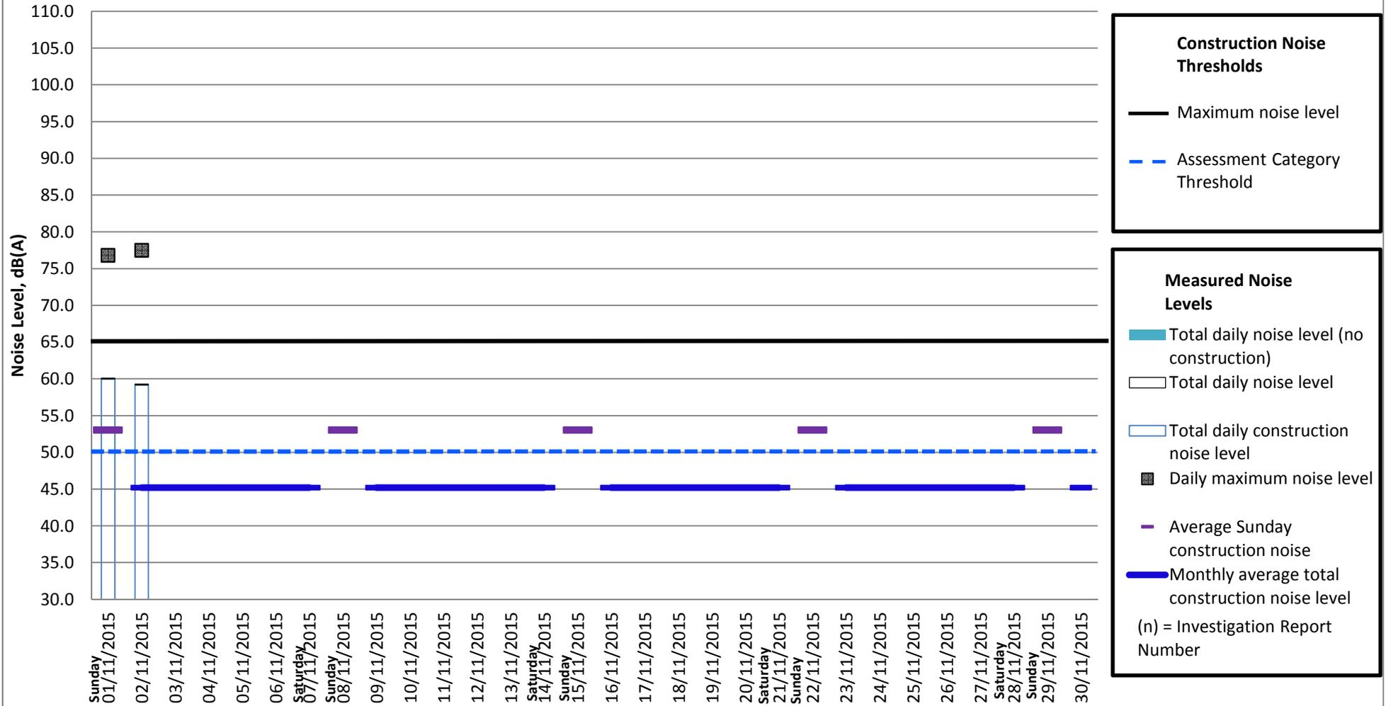
**Construction Noise Thresholds**
