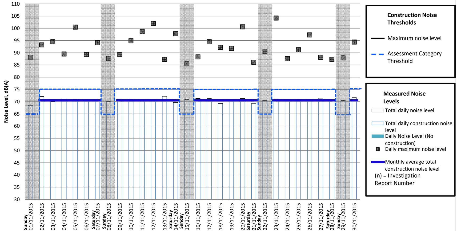
**Note:** The grey areas of the chart represent days on which no construction works have been conducted. It should be noted that the measured noise levels Mon - Fri can not be attributed to construction works due to the considerable distance (1.75 kilometers) between this monitoring location and the closest construction works.
