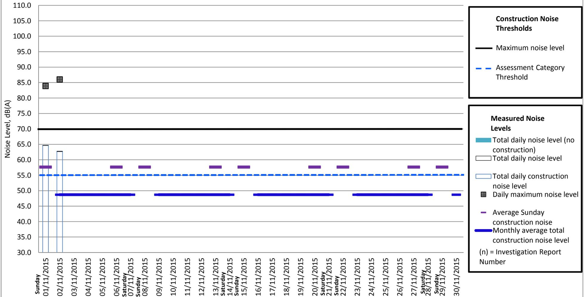
**Note:** Note; The B800 bridge demolition took place over from 31/10/2015 at 22:00 until 02/11/2015 at 07:00. Noise levels have been included if for this month
