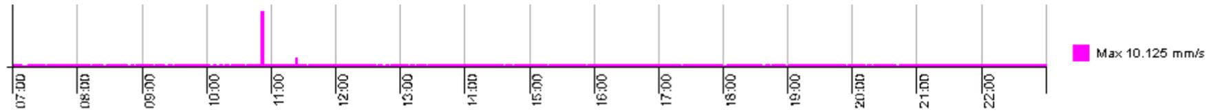
Exceedance on the 13/07/2015 has been investigated and found not to be construction related. Due to the intervening distance between the works and the Springfield monitor, a vibration level of such magnitude would also be expected to have been picked up on other monitors in that area i.e. Clufflat and Linn Mill. Subsequent analysis revealed no such similarities for the time period in question.
