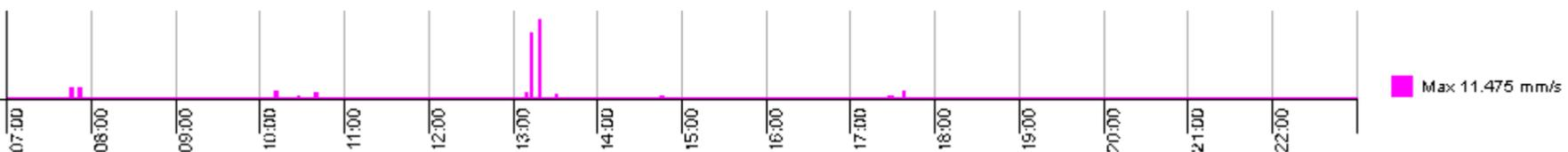
Exceedance on the 21/08/2015 has been investigated and found to be an isolated event with no similar exceedances at that time on the surrounding vibration monitors. Investigations also found no construction related exceedances at that time on the noise monitor at Linn Mill which is 45 meters closer to the construction site
