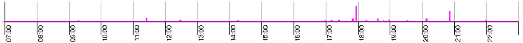
Exceedances on the 2<sup>nd</sup>, 4<sup>th</sup>, 7<sup>th</sup> and 8<sup>th</sup> of December have been investigated and found to be either intermittent or one off isolated events in which the source of the vibration could not be determined. It is highly unlikely to have been caused by construction related activities (graph above from the 08/12/2015). There is however, works ongoing at the property where the vibration monitor is sited, which could be causing the intermittent vibration levels.
