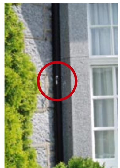
The monitors collect nitrous oxide (NO<sub>2</sub>) from the air, which is an air pollution indicator. Once collected the tubes are sent to a lab for analysis of the levels of NO<sub>2</sub> in the air during that monthly period.
