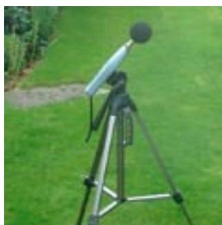
The short term monitoring survey involves setting up the equipment and monitoring the noise levels for 30 minutes, removing the equipment and then revisiting the site a number of times during the same day and repeating the process a number of times. The equipment is not left unattended at any time.
