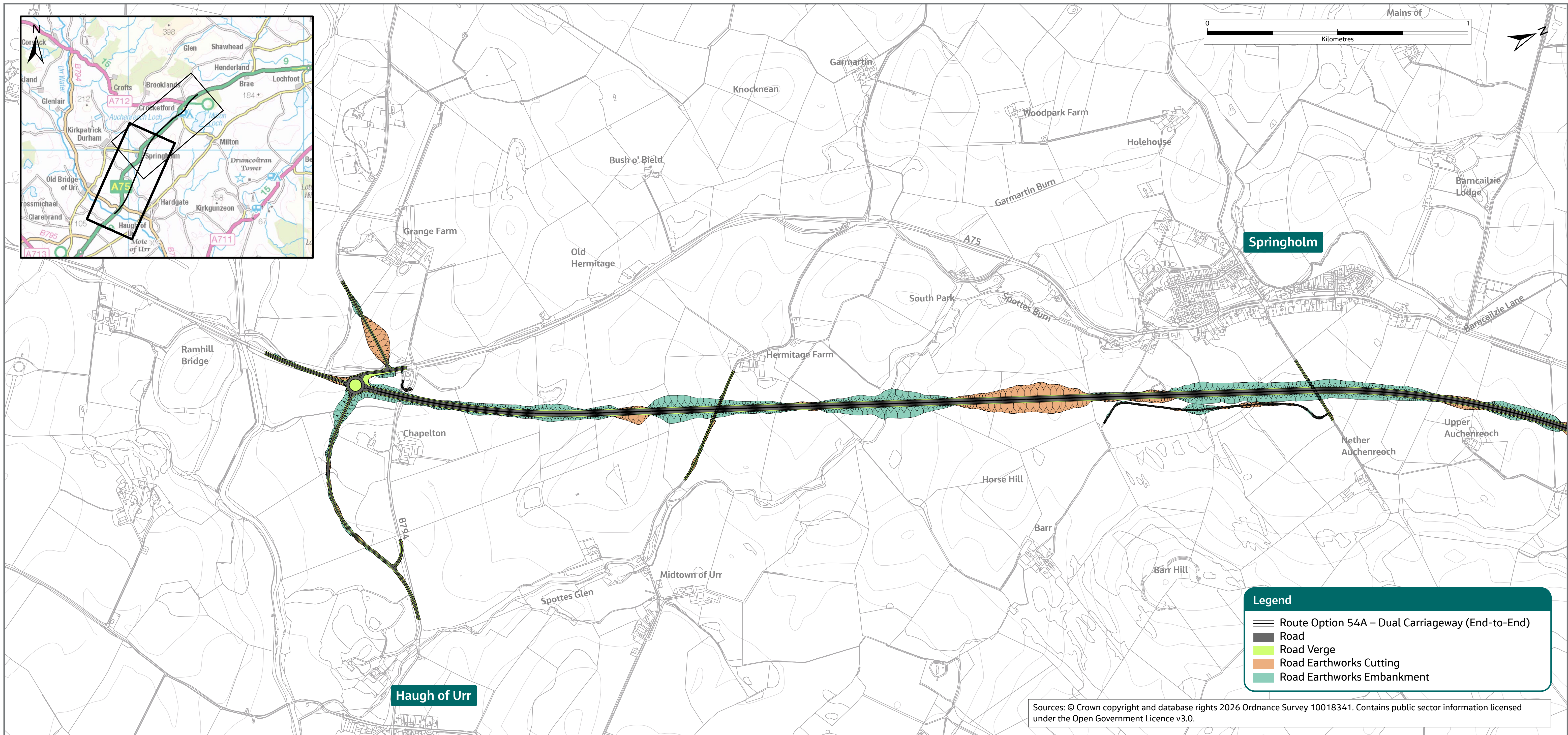
Dual carriageway (end-to-end) route option 54A from Urr Water to Larglea southern extent
