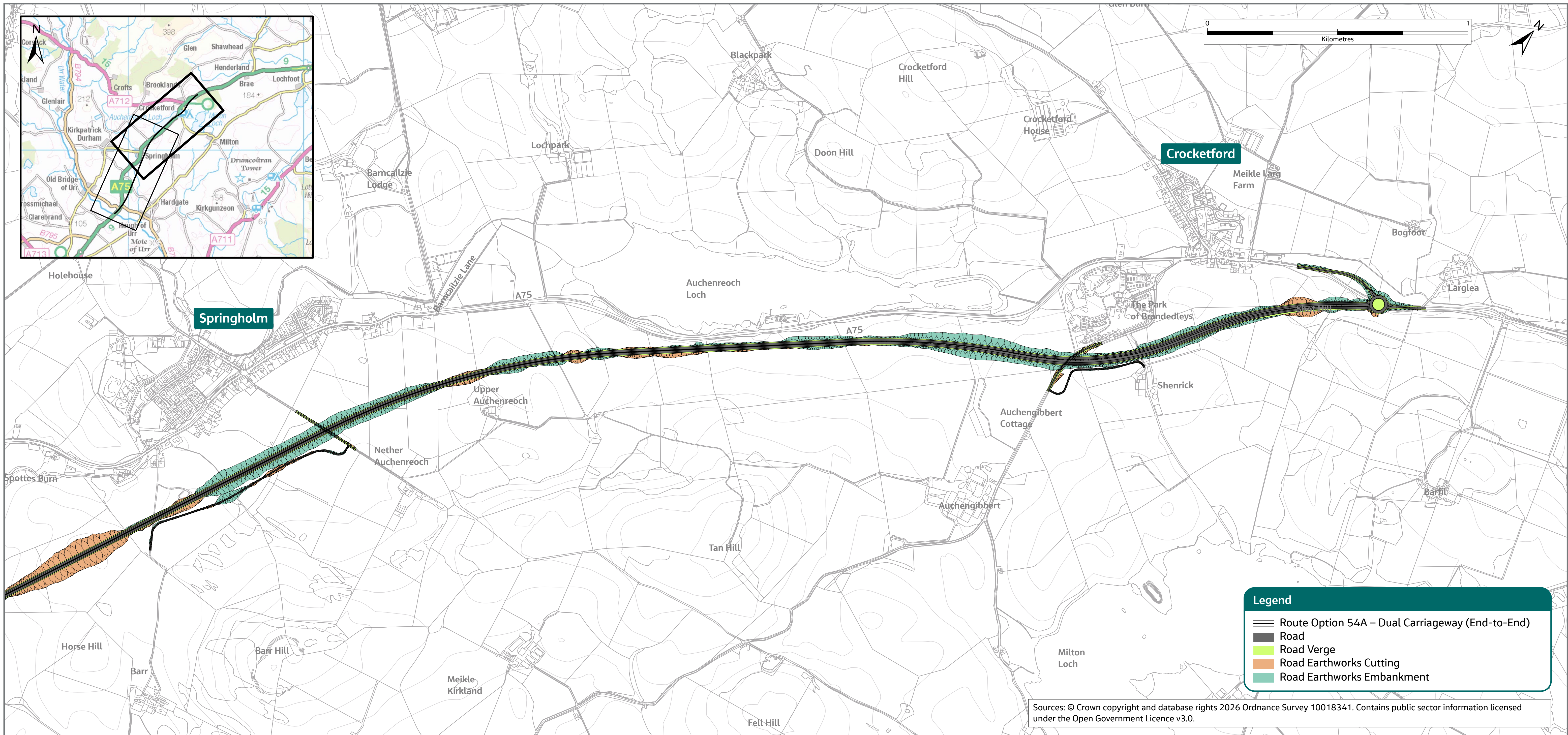
Dual carriageway (end-to-end) route option 54A from Urr Water to Larglea northern extent
