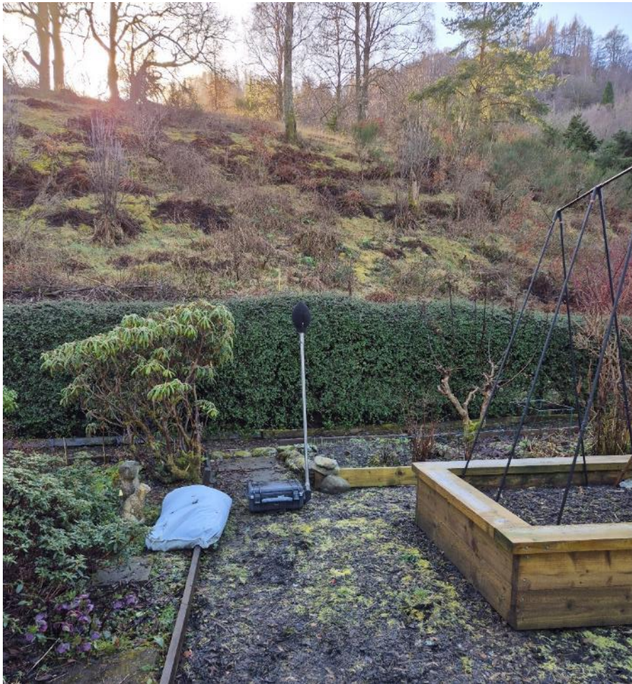
Photograph A15.2-2: Noise Monitoring Equipment at Hollybank
