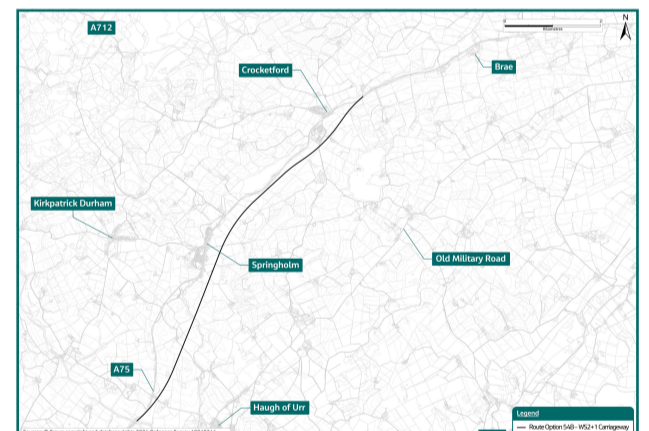
Route Option 54B (WS2+1 carriageway, end-to-end): Urr Water to Larglea. Sifted out following Cross-section Assessment
